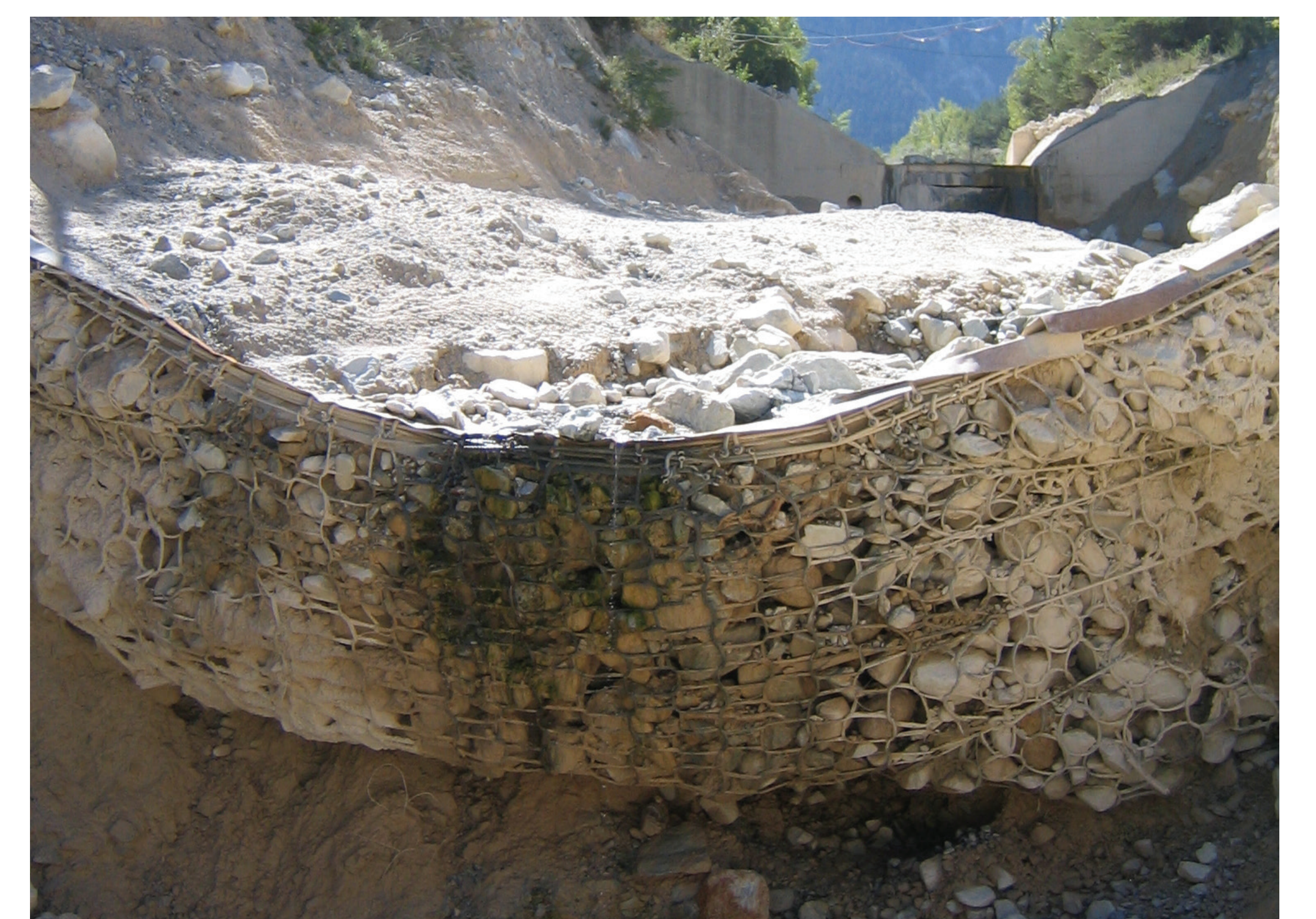
Test in Illgraben/Switzerland, retention capacity approx. 1000 m³
